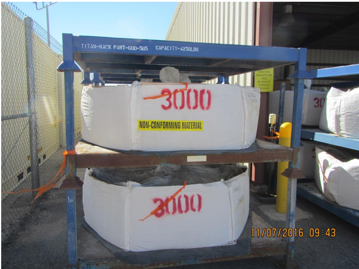
Figure 4: Non-conforming MgO Awaiting Testing and Repackaging
